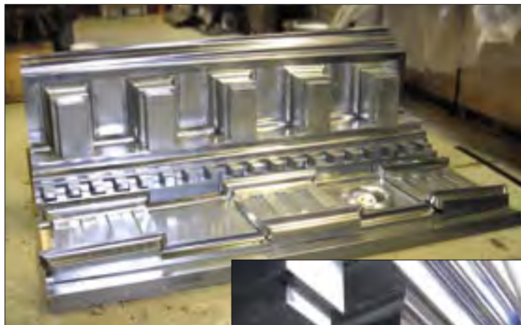
Seventy years of wind and weather had compromised the intricate beauty of 40 Tiemann’s distinctive metal cornices. Craftsmen from Michigan Ornamental fabricated 144 lineal feet of design-enhanced replacements to restore the building’s original elegance.
